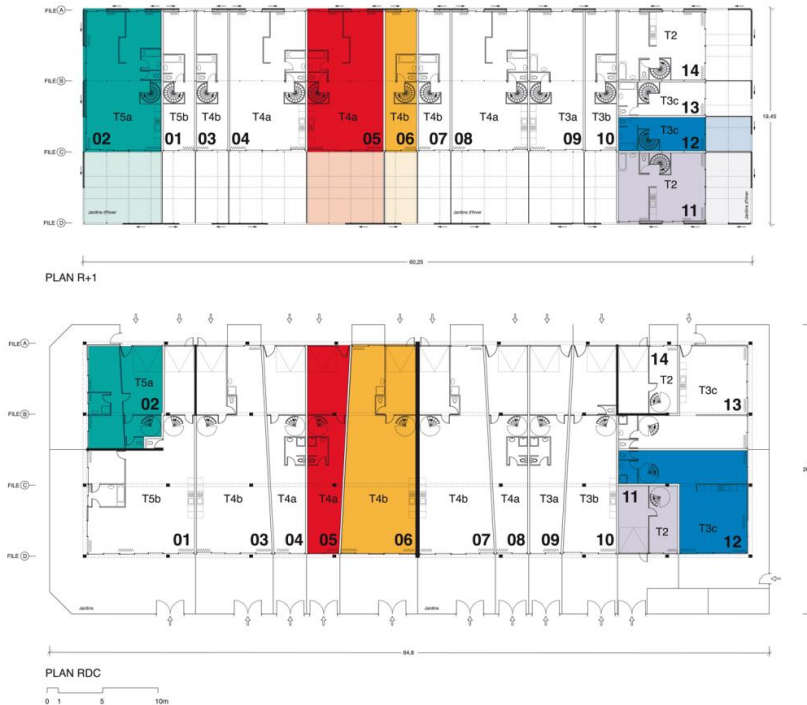
Houses in Mulhouse – Plans: Ground floor and first floor. The area of one colour show the floor area of one apartment. Source: www.lacatonvassal.com
