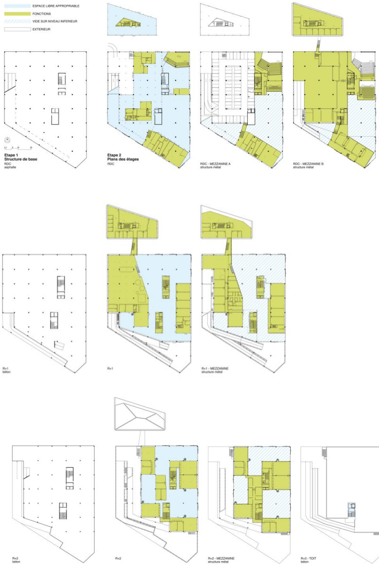
Nantes Architecture School – Plans: starting from ground floor up to the roof. Programmed space is coloured olive green, functionally non-assigned floors light blue, and outdoor floors are white. Source: www.lacatonvassal.com
