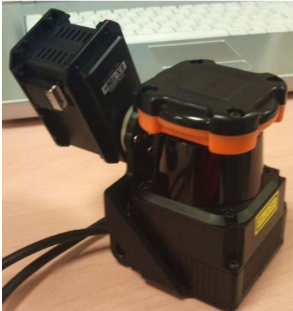
Fig. 1. Prototype based on Hokuyo range-finder attached to a Dynamixel servomotor.
