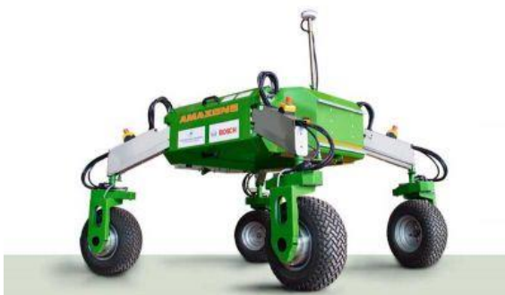
Amazone-Bosch BoniRob lightweight field robot
