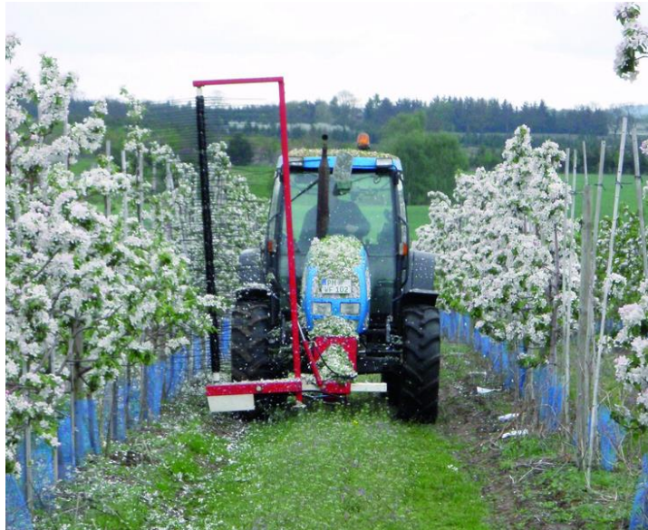
DARWIN blossom thinner equipped with a camera system and in action in an apple orchard.
