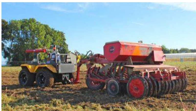
Clearpath Grizzly RUV pulling implement
