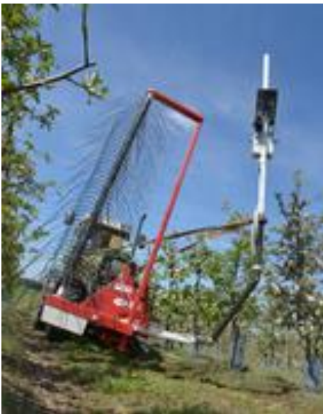
DARWIN blossom thinner equipped with a camera system and in action in an apple orchard.
