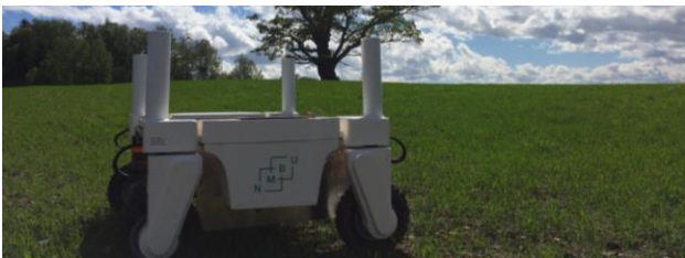
Thorvald, multiple-purpose lightweight agricultural robot
