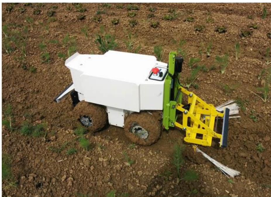
Oz, the electric hoeing robot
