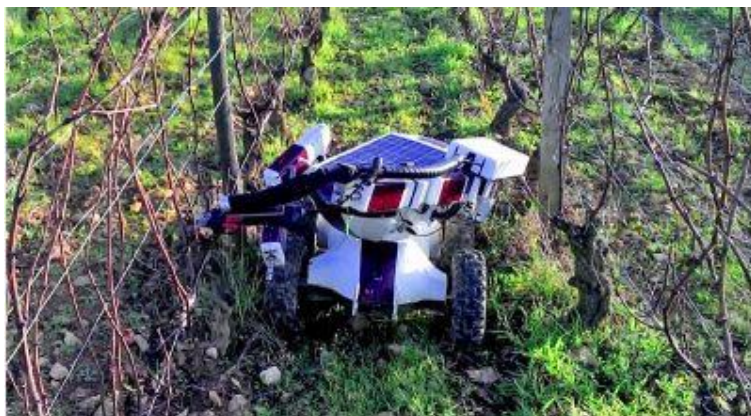
Wall-Ye 1000 pruning robot in a vineyard.
