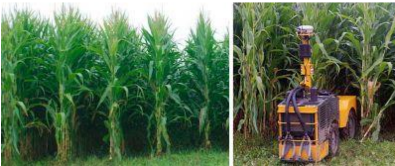
Rowbot in cornfield. Rowbots work in teams to apply nitrogen fertilizer in sync with precision needs
