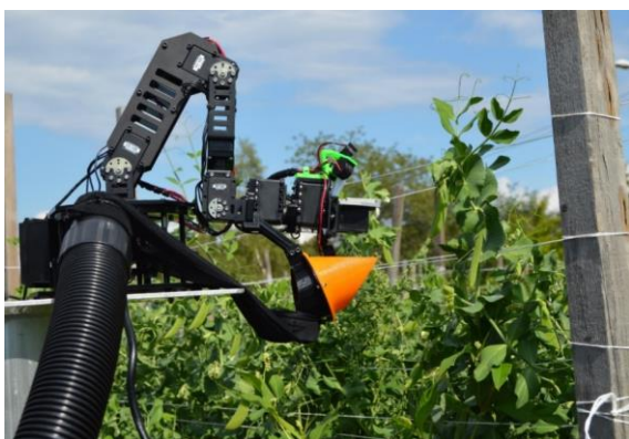
Robot for harvesting sugar snap peas
