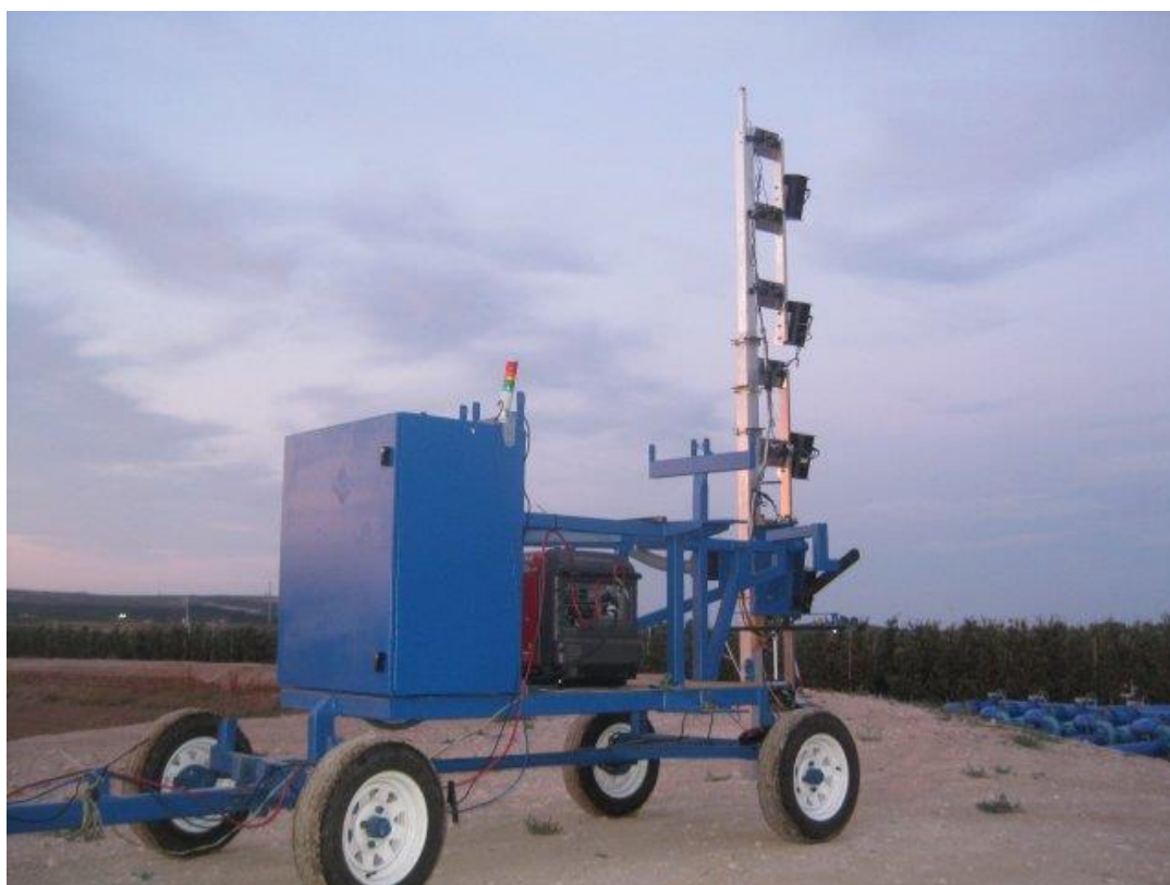
Vision Robotics crop load estimation
